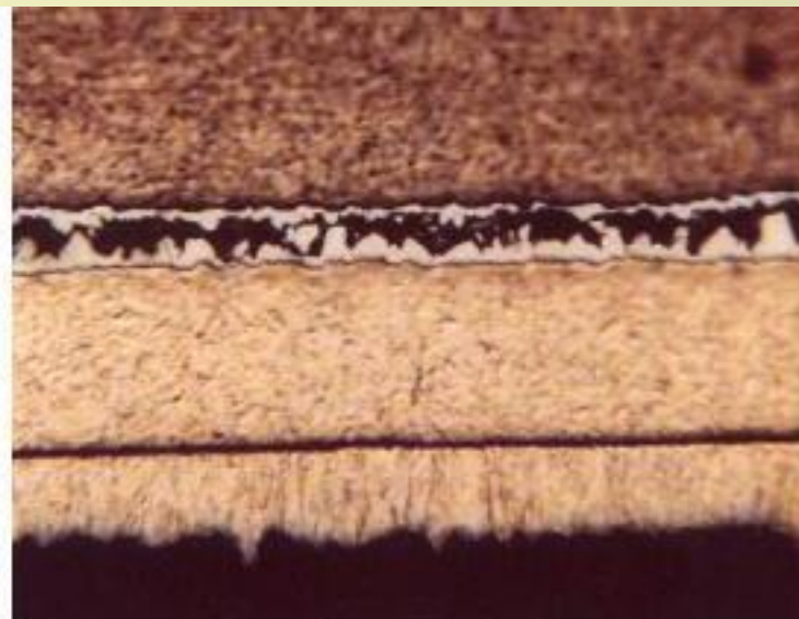
Figure 9- Buildup of weak Pb-rich phase (Dark areas in microstructure) as a result of Sn depletion through reaction with Au and Ni.
