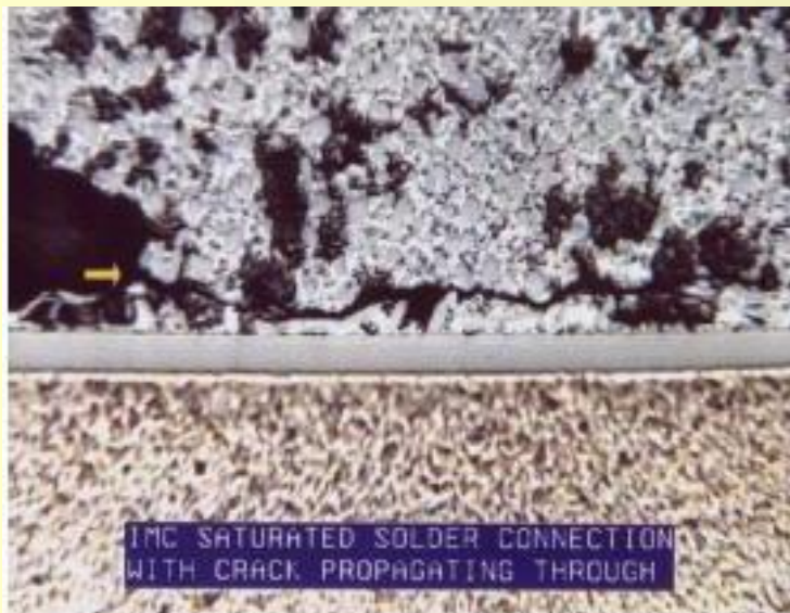
Figure 10- Crack propagating through IMC saturated solder connection.
