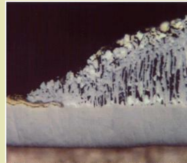
Figure 8-Concentrated Au-Sn IMC at leading edge of Solder as it reacts with Au deposit.
