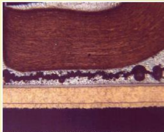
Figure 12-Outgassing from Au plating in confined space that has resulted in aligned voids between two flat mating surfaces.
