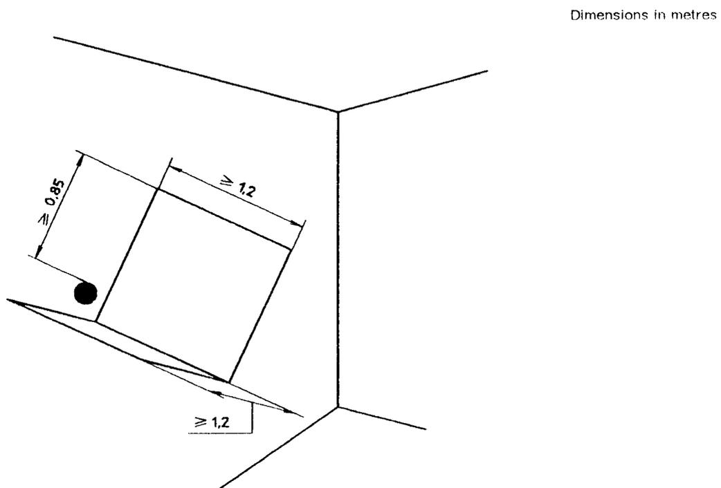
**Figure C.1 — Drawing showing in principle how to simulate a corner position by attaching reflective panels at right angles to the partition wall mounted in the test opening**
