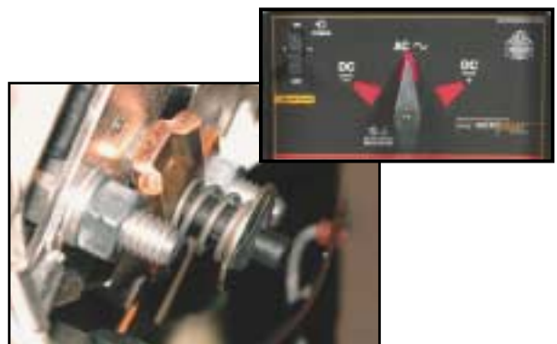
Snap-action durable switches make positive mechanical contact to reduce chances of intermittent contact failure.
