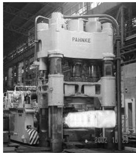
3000 ton Open Die Forging Press 25 ton railb. Manipulator 16 ton railb. Manipulator
