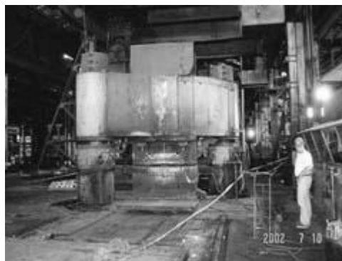
5000 US-ton hydraulic Open Die Forging Press(New single cylinder crosshead (was 3-cylinder crosshead))
