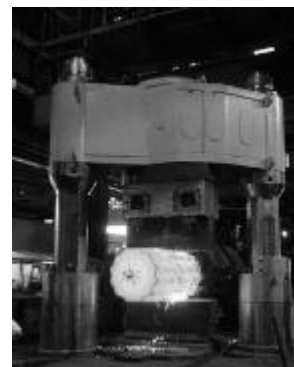
5000 US-ton hydraulic Open Die Forging Press(New single cylinder crosshead (was 3-cylinder crosshead))
